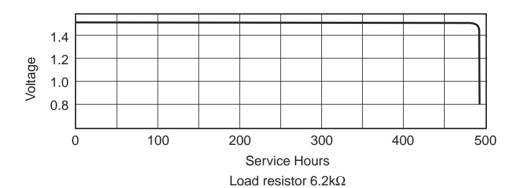
Average Service Capacity: 120 mAh (rated capacity at  $6.2k\Omega$  load, cut off voltage 1.2V at  $20^{\circ}C$ )
