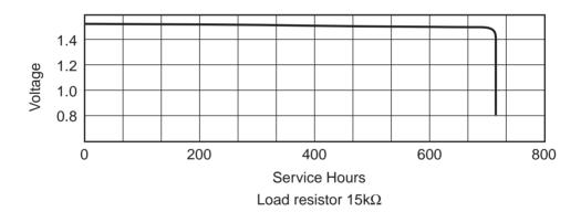
Average Service Capacity: 70 mAh (rated capacity at  $15k\Omega$  load, cut off voltage 1.2V at  $20^{\circ}$ C)
