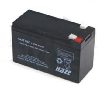
Chemistry: Sealed Lead Acid Volts: 12 Volt Batteries Amp Hours: 8 AH with T2 Insert Terminals Description: RBC 51 Equivalent is 1 x 12V 8 AH batteries Weight: 5.25lbs.
